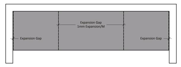
To secure evostone, apply liberal dabs of silicone every 150-200mm to the top edges of the cabinets. Support the Evostone when lowering into position. DO NOT SCREW INTO EVOSTONE
