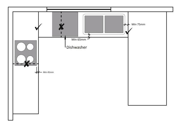
Freestanding cookers must be installed so the level of the hob is not below the benchtop and allow clearances as recommended by the appliance manufacturer or a minimum of 2mm, whichever is the greatest.
