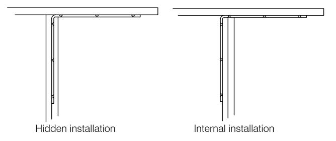
Spacing of bracket must not exceed 900mm and 300mm from the end of the benchtop.
